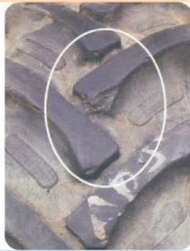
Chipping/ Tearing of Leading Edges
