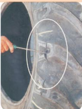
Circum- ferential Cracks at Buttress
