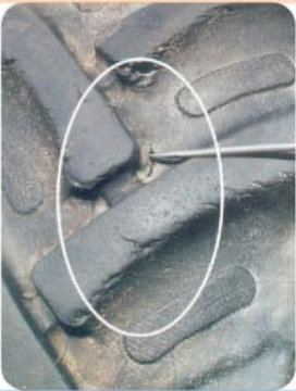
Lug base cracks/ Tie bar Cracks
